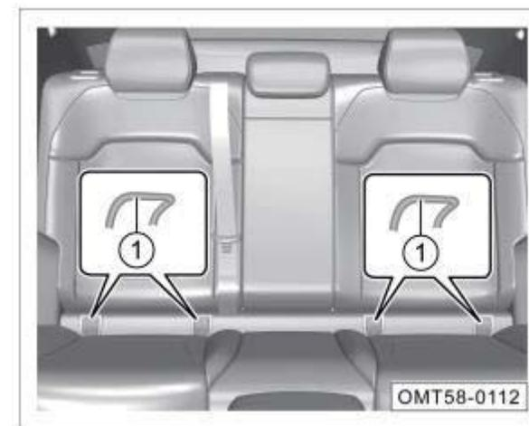
Open the cover, and you can see that the front anchorage ① of the rear seat is under the cover.
