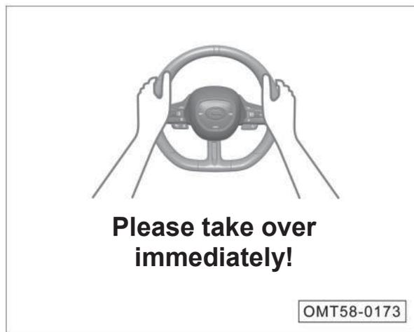
When the LDW detects that the driver's hands are off the steering wheel for a long time, the system will issue a hands-on reminder, and the ICM will display the above figure with an audible alarm. This reminder only exists if the driver selects "Steering" or "Steering and warning".
