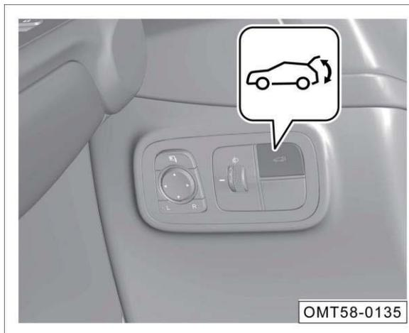
Press and hold the liftgate button on the instrument panel to open the liftgate.
