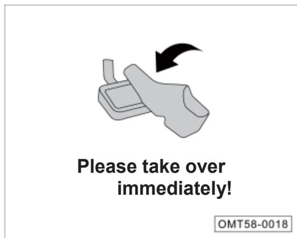
The ICA system can only use the limited braking capacity of the service brake system. When the system requires the driver to intervene in braking, the ICM will display the above figure and the buzzer will sound.
