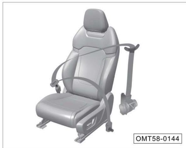
In the event of a car collision, fastening seat belts correctly can restrain the driver and passengers in a proper position and slow down the inertia of their forward movement, thus preventing them from being thrown forward, and at the same time enable them to get the best protection from the airbag, thus reducing their impact injury as much as possible.
