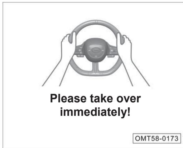
When ICA detects that the driver's hands are off the steering wheel for a long time or detects that the vehicle reaches the control limit (curve) and there is a risk of crossing the lane, the ICM will display the above figure and the buzzer will sound.
