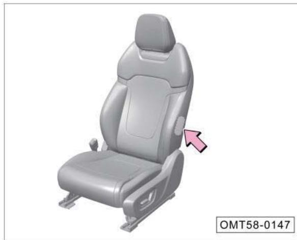
Front and rear side airbags are installed on the outside of the front seat and rear seat (as indicated by the dotted shaded area) marked with "AIRBAG".
