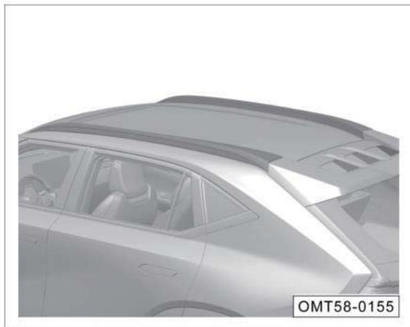
The roof rack equipped on this vehicle is a decorative part and cannot directly bear articles.
