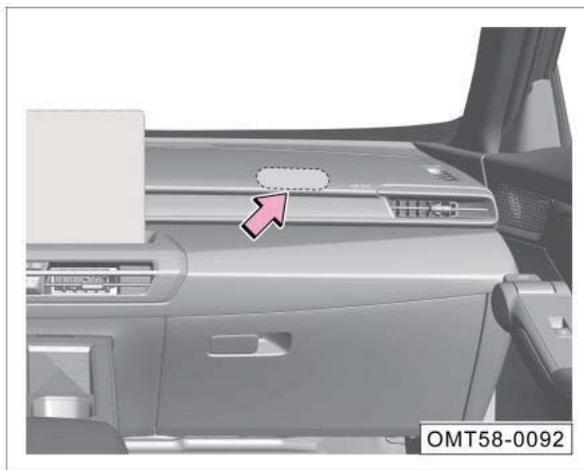
The front passenger's frontal airbag is installed inside the instrument panel (as indicated by the dotted shaded area) marked with "AIRBAG".
