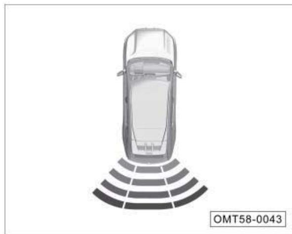
The dynamic view on the display indicates the distance between the current vehicle and the obstacle. In the view, the outermost layer of the vehicle is green line, and the inner layer gradually becomes yellow line, orange line and red line. When the obstacle is getting closer and closer to the vehicle, the color line will gradually change from the outermost layer to the inner layer.
