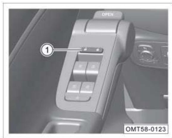
The central locking control button ① can be used to lock and unlock the doors in the car:
