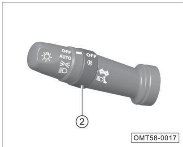
When START/STOP button is in the "ON" position with the low beams turned on, turn the fog lamp switch ② to turn on or off the
