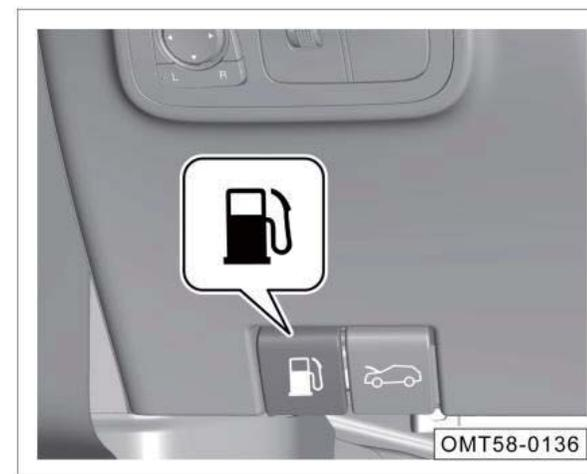
1. Pull up the fuel tank cap release handle
