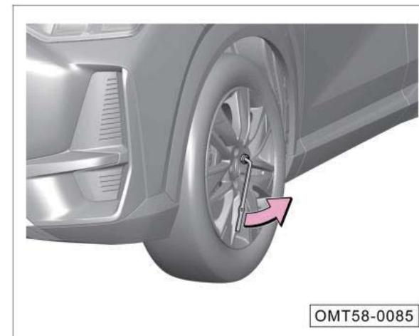
Set the wheel bolt removal wrench firmly on the wheel bolt, and loosen the wheel bolts counterclockwise.
