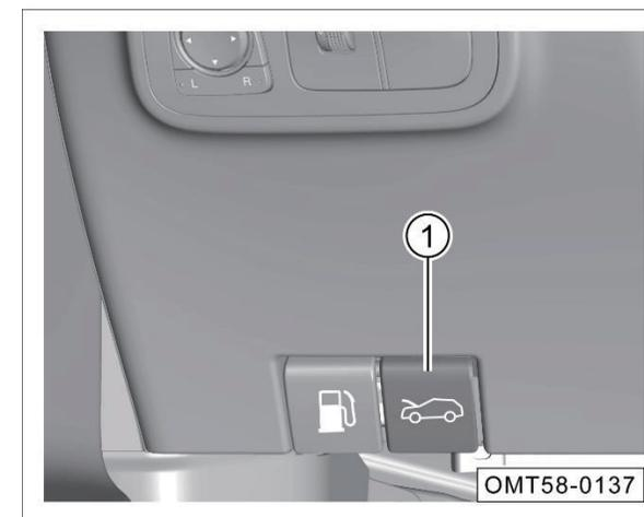
1. Pull the hood release handle ① to unlock the hood and make it bounce slightly.
