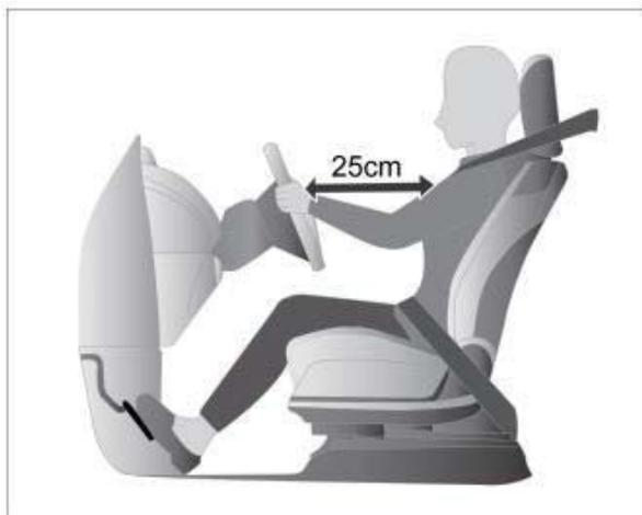
1. Adjust the driver's seat to a suitable position to ensure that the distance between the steering wheel and your chest is not less than 25 cm.
