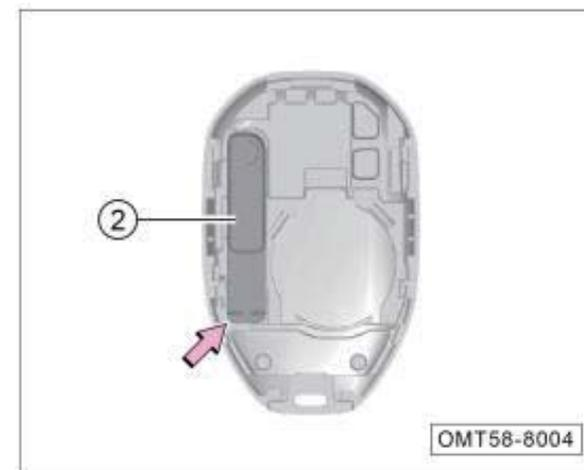
2. Pick up the emergency mechanical key ② as arrowed.
